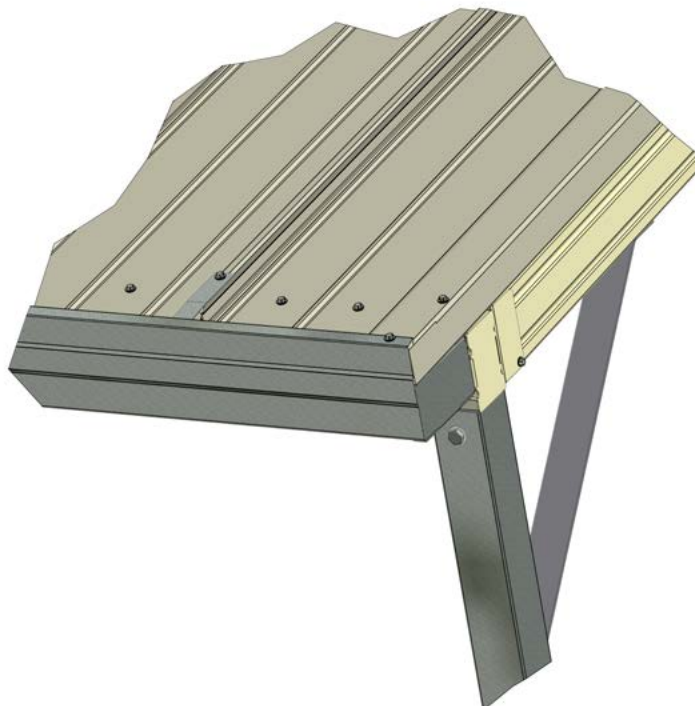
Finished Gutter Assembly - Non-Downpipe End
