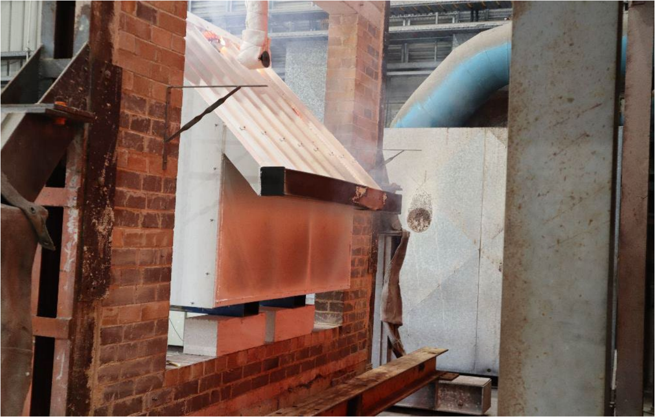
PHOTOGRAPH 7 – EXPOSED FACE OF SPECIMEN DURING 16 KW/M 2 EXPOSURE
