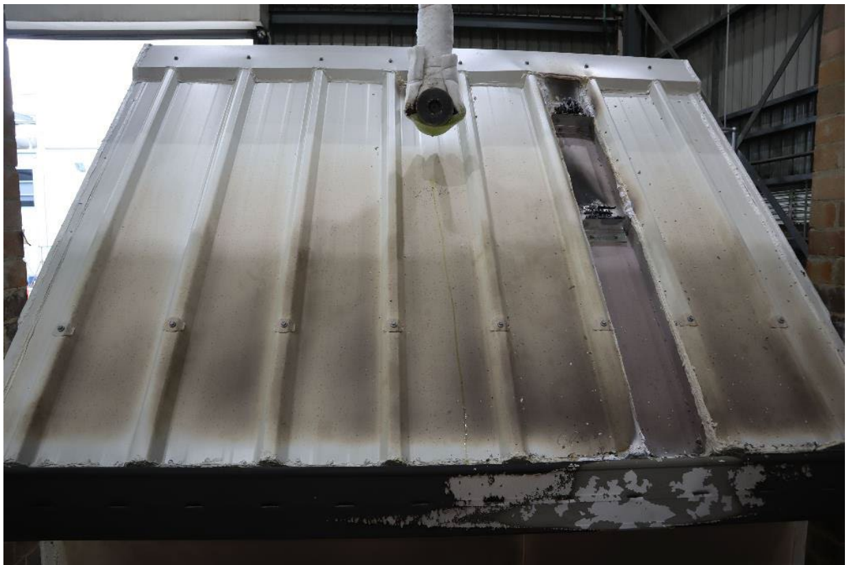
PHOTOGRAPH 12 – EXPOSED FACE OF SPECIMEN AT 15 MINUTES INTO THE TEST
