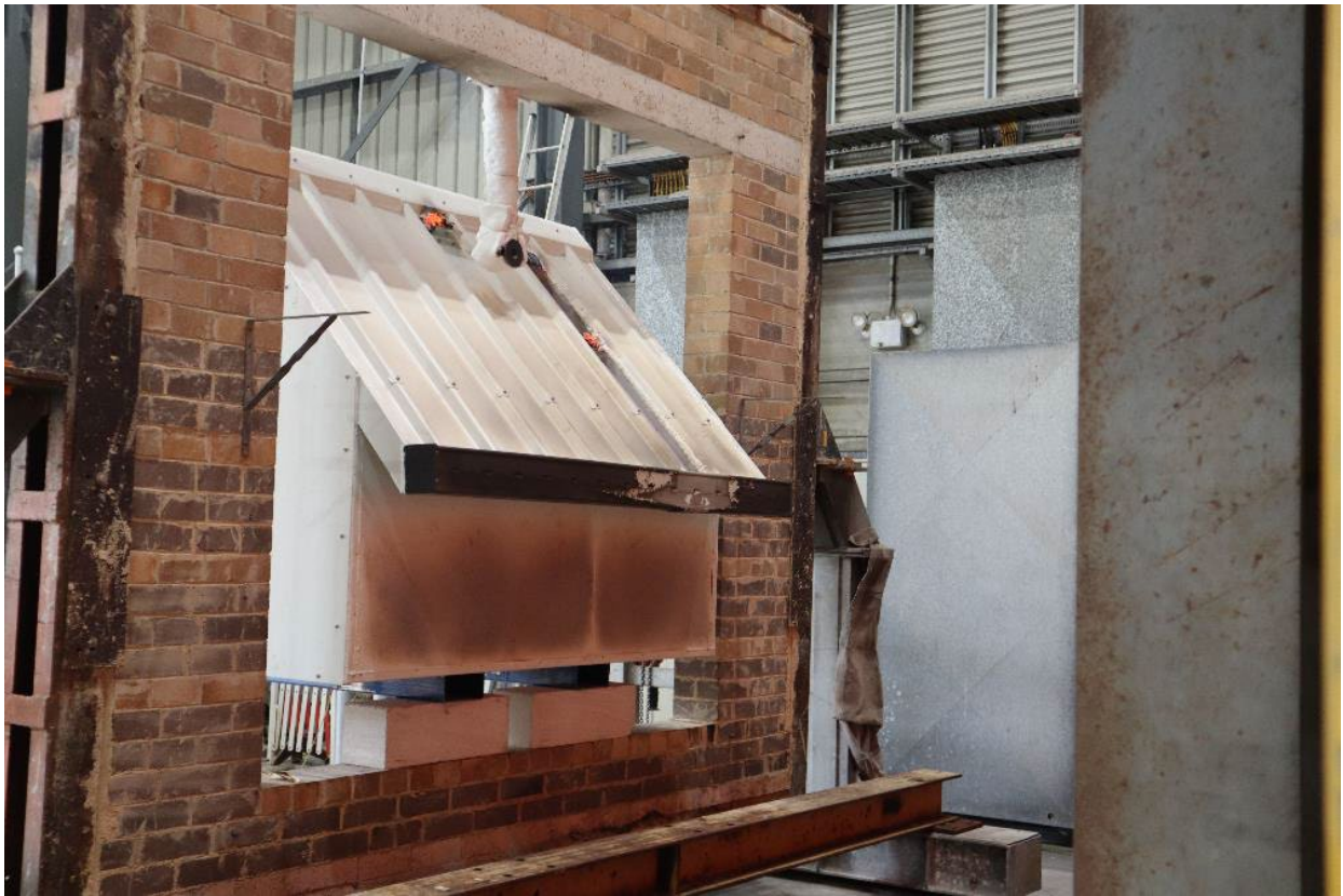
PHOTOGRAPH 11 – EXPOSED FACE SPECIMEN AT 5 MINUTES INTO THE TEST
