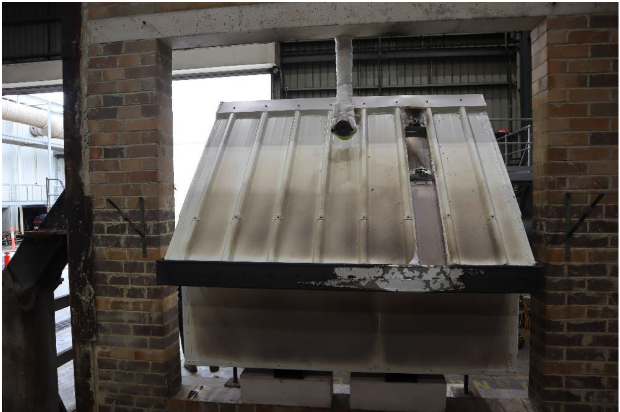
PHOTOGRAPH 15 – EXPOSED FACE OF THE SPECIMEN AT THE CONCLUSION OF TESTING
