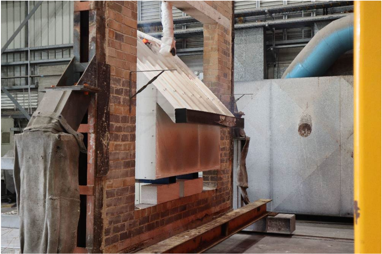
PHOTOGRAPH 9 – EXPOSED FACE OF SPECIMEN DURING 8.5 KW/M 2 EXPOSURE
