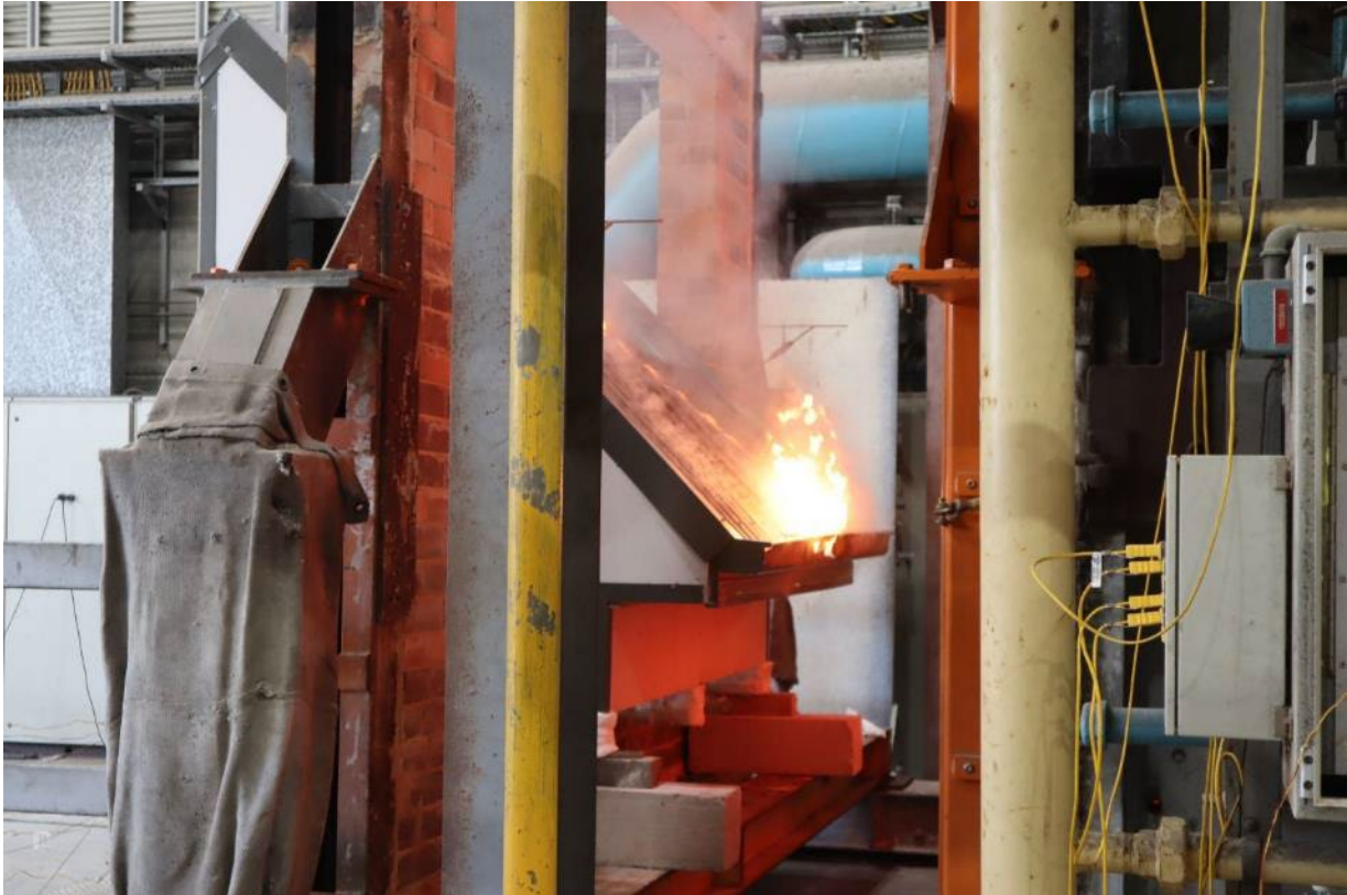
PHOTOGRAPH 5 – EXPOSED FACE OF SPECIMEN DURING 29 KW/M 2 EXPOSURE
