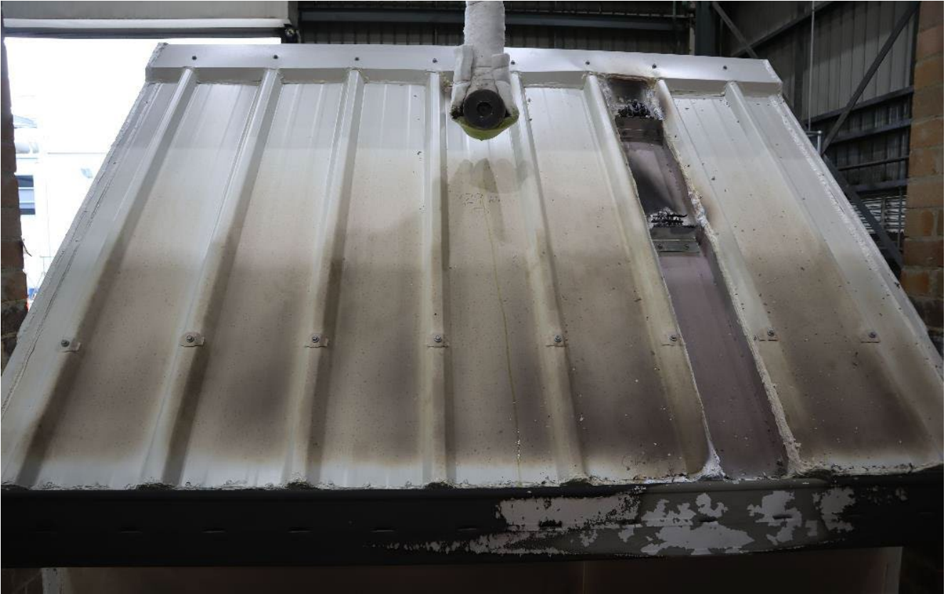
PHOTOGRAPH 13 – EXPOSED FACE OF SPECIMEN AT 15 MINUTES INTO THE TEST
