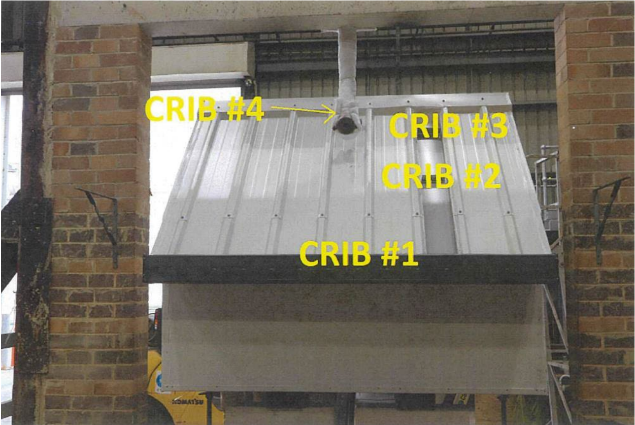
PHOTOGRAPH 4 – EXPOSED FACE OF THE SPECIMEN SHOWING CRIB LOCATIONS PRIOR TO TESTING
