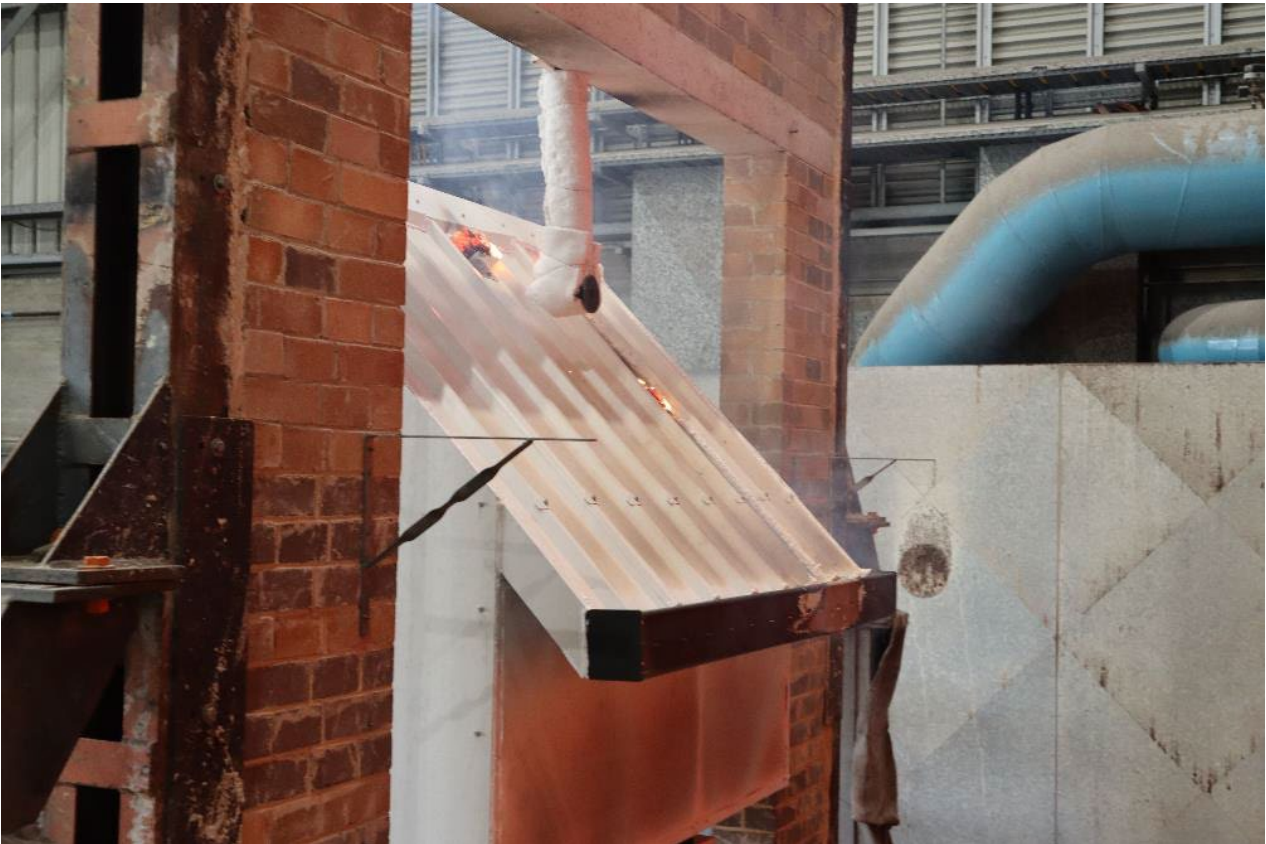
PHOTOGRAPH 8 – EXPOSED FACE OF SPECIMEN DURING 12 KW/M 2 EXPOSURE
