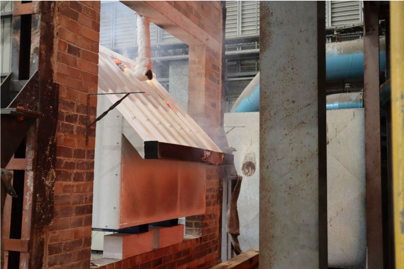
PHOTOGRAPH 6 – EXPOSED FACE OF SPECIMEN DURING 24 KW/M 2 EXPOSURE
