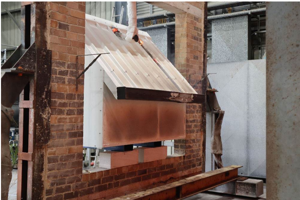
PHOTOGRAPH 10 – EXPOSED FACE OF SPECIMEN DURING 7 KW/M 2 EXPOSURE
