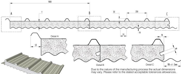
DeltaTrimCorro-EPS-FR is an Insulated Roof Panel System, comprising of two pre-painted, roll-formed steel skins, bonded to a fire retardant grade expanded polystyrene insulating core.
