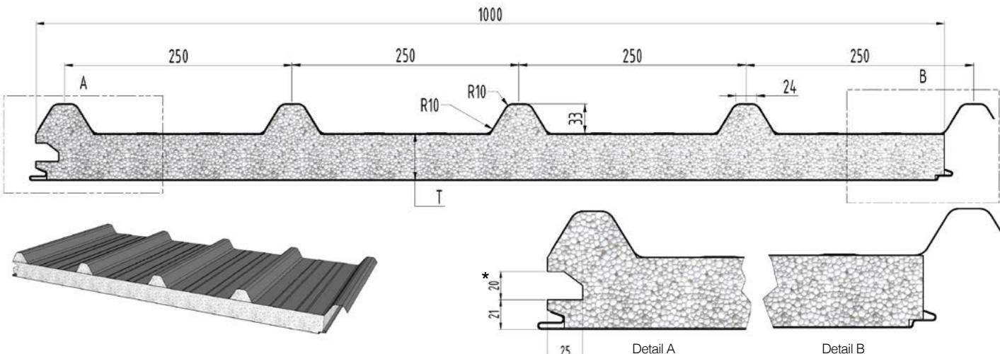
**DeltaTrim-EPS-FR** is an Insulated Roof Panel System, comprising of two pre-painted, roll-formed steel skins, with a fire retardant grade expanded polystyrene insulating core.
