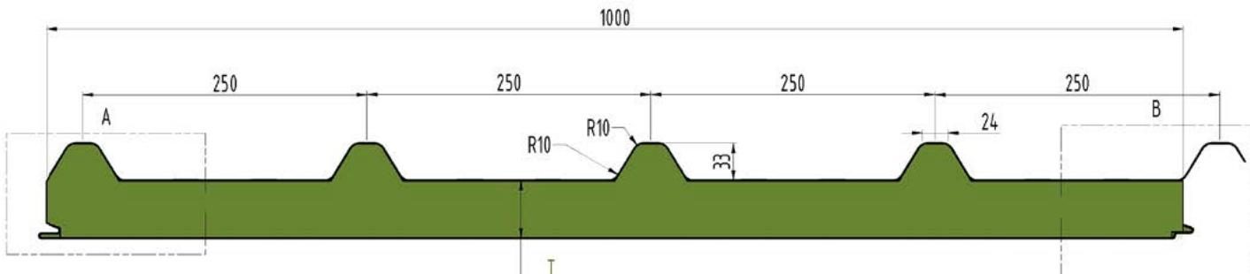
**DeltaTrim-MW** is an Insulated Roof Panel System, comprising of two pre-painted, with roll-formed steel skins bonded to a non-combustible mineral wool core.
