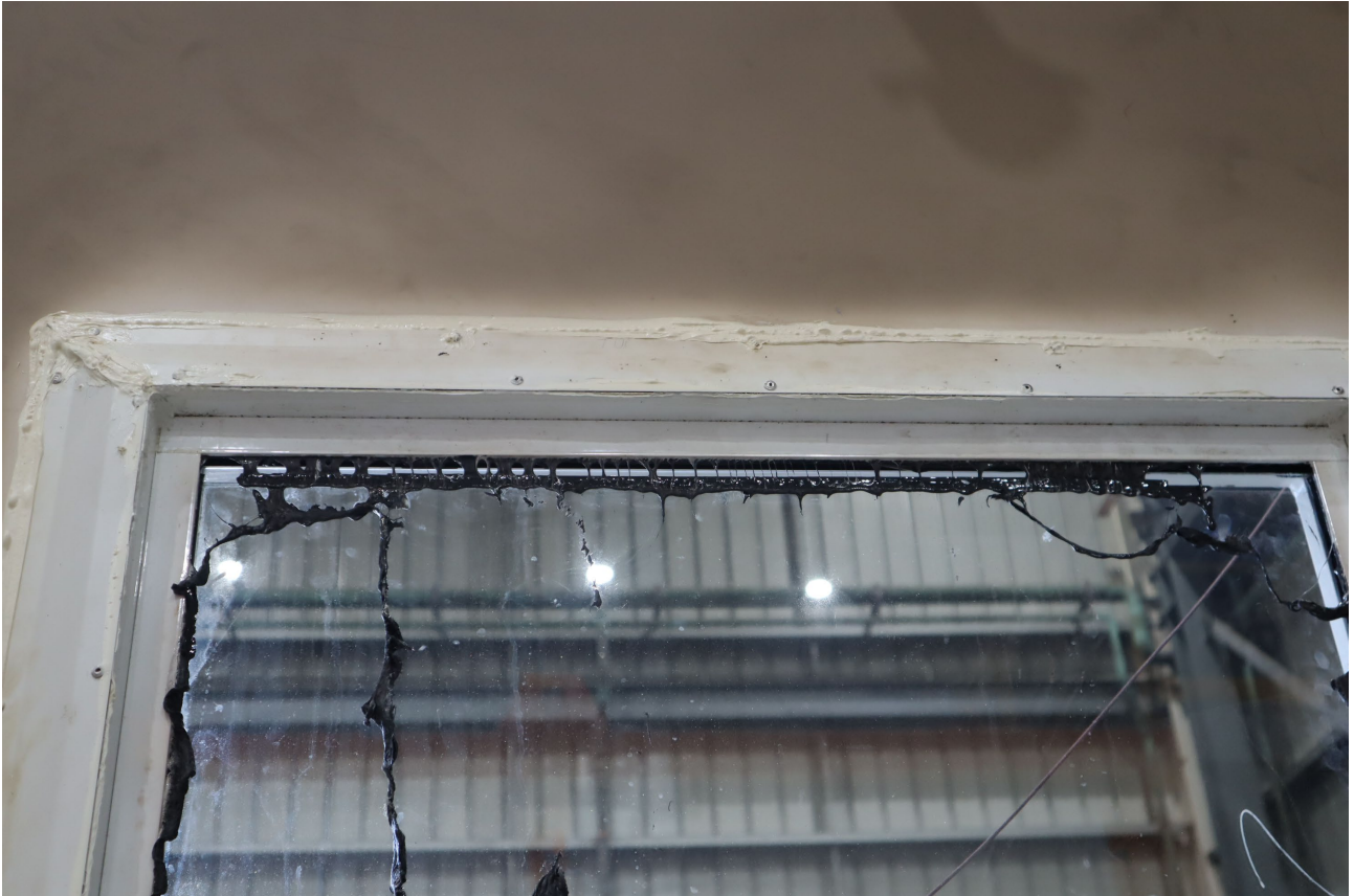
PHOTOGRAPH 16 – EXPOSED FACE OF THE SPECIMEN AT 16 MINUTES INTO THE TEST
