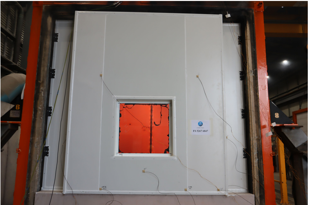
PHOTOGRAPH 13 – UEXPOSED FACE OF THE SPECIMEN AT 7 MINUTES INTO THE TEST
