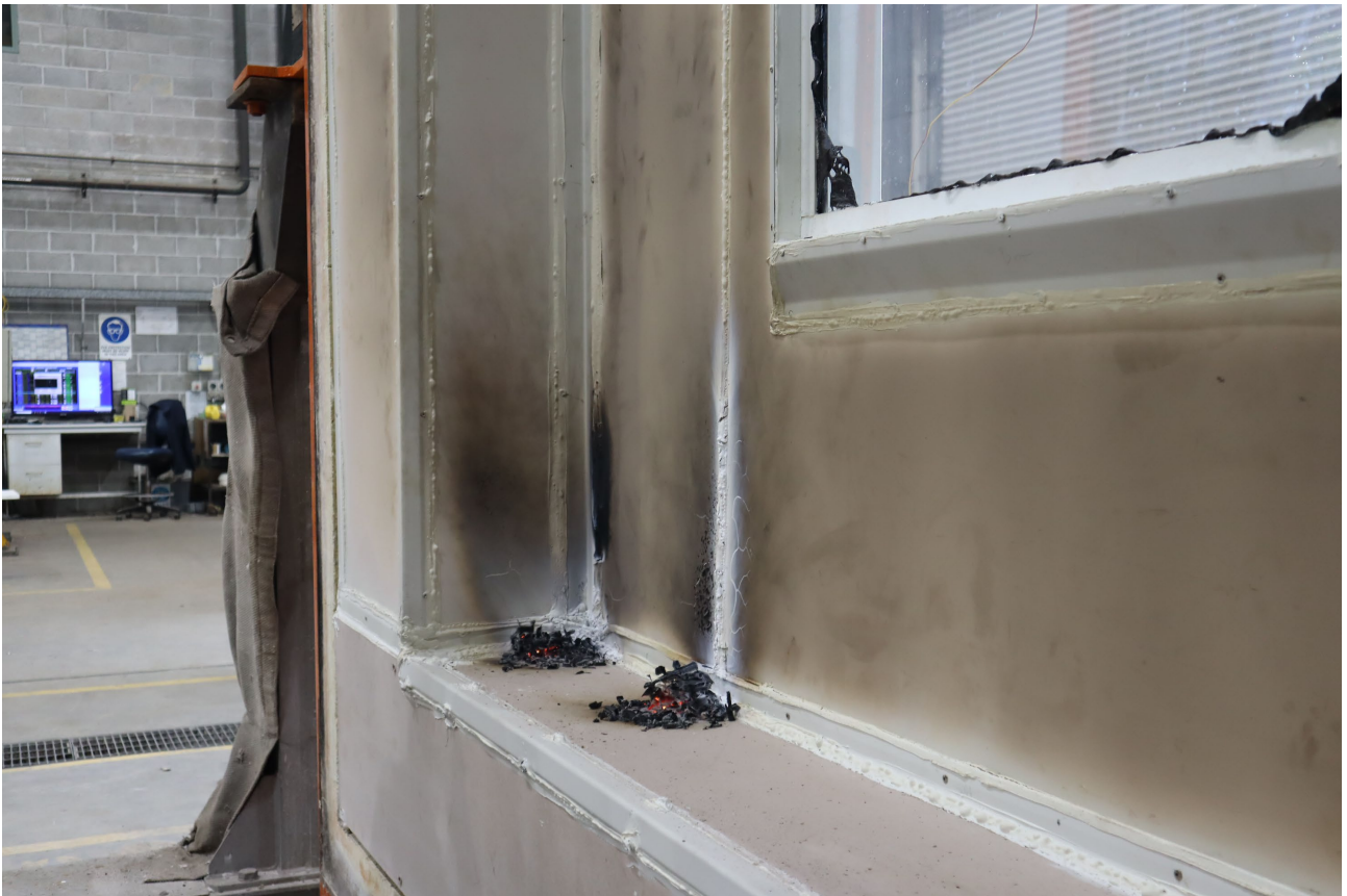
PHOTOGRAPH 15 – EXPOSED FACE OF SPECIMEN AT 12 MINUTES INTO THE TEST
