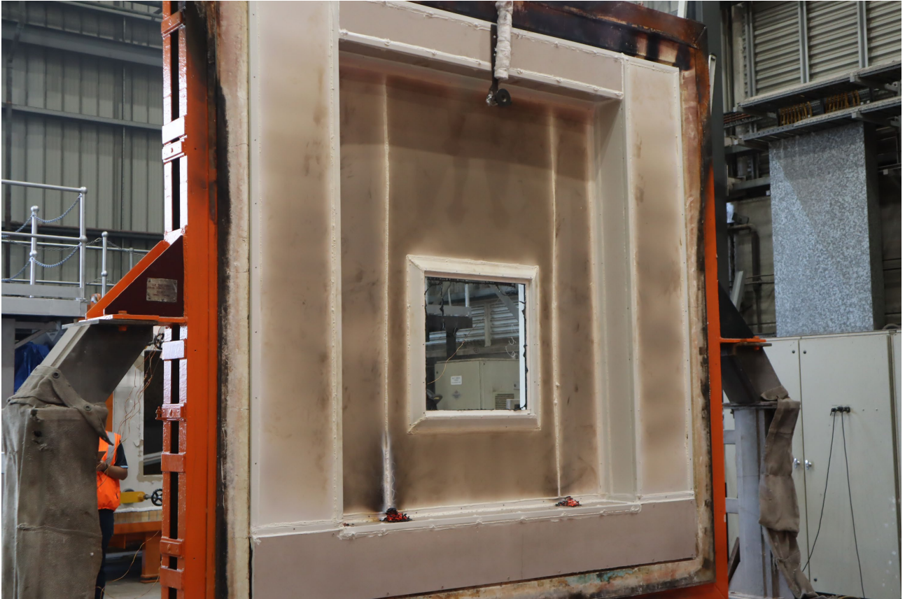
PHOTOGRAPH 14 – EXPOSED FACE OF THE SPECIMEN AT 7 MINUTES INTO THE TEST
