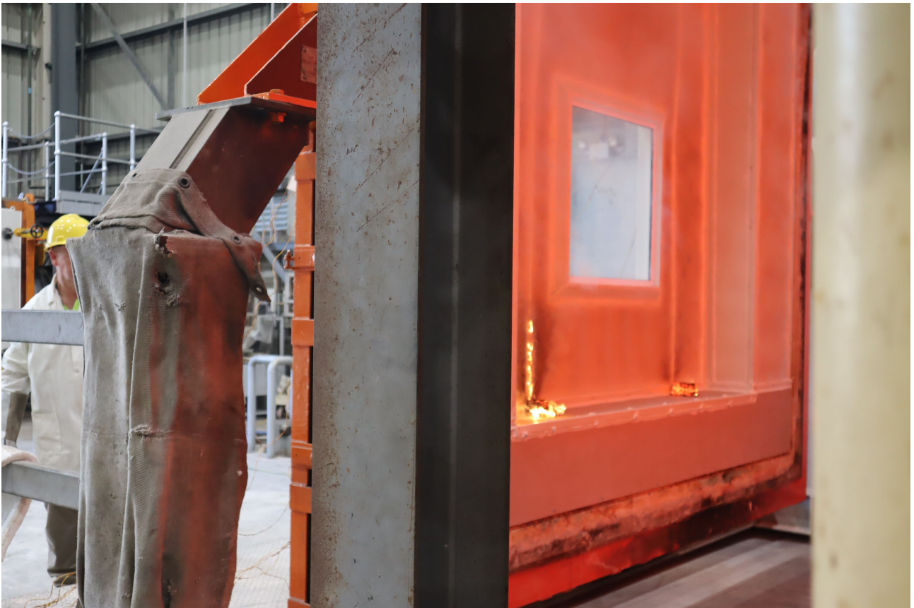
PHOTOGRAPH 9 – EXPOSED FACE OF SPECIMEN DURING 21 KW/M 2 EXPOSURE
