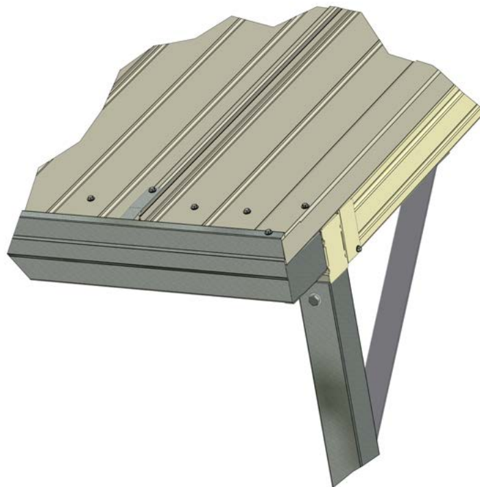
Finished Gutter Assembly - Non-Downpipe End
