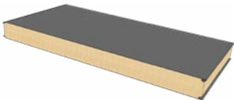
DeltaCool™ is an Insulated Wall Panel System, comprising of two pre-painted, roll-formed steel skins, bonded to an insulated core of either fire retardant grade polystyrene, polyisocyanurate, thermosetting phenolic composite or mineral wool.
