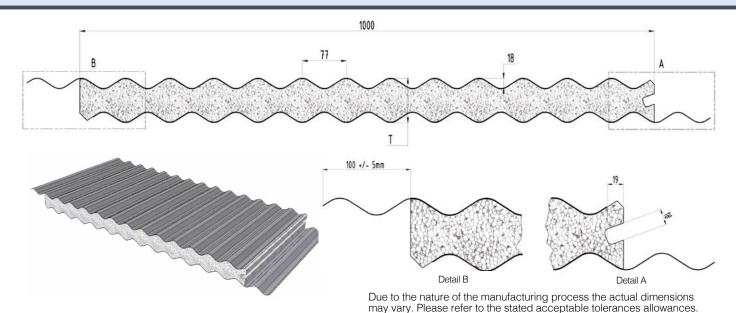
DeltaCorroCorro-EPS-FR is an Insulated Roof Panel System, comprising of two pre-painted, roll-formed steel skins, bonded to a fire retardant grade expanded polystyrene insulating core.
