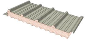
**DeltaTrimCorro-TPC** is an Insulated Roof Panel System, comprising of two pre-painted, roll-formed steel skins, bonded to a thermosetting phenolic composite insulating core.
