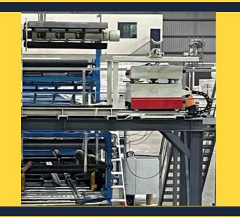
To improve the consistency of the flatness of steel finish on the under skin on our range of DeltaTrim ® & DeltaOrb ® roof panels we have installed a new upgraded feed-in section to our continuous roof laminating machine.
